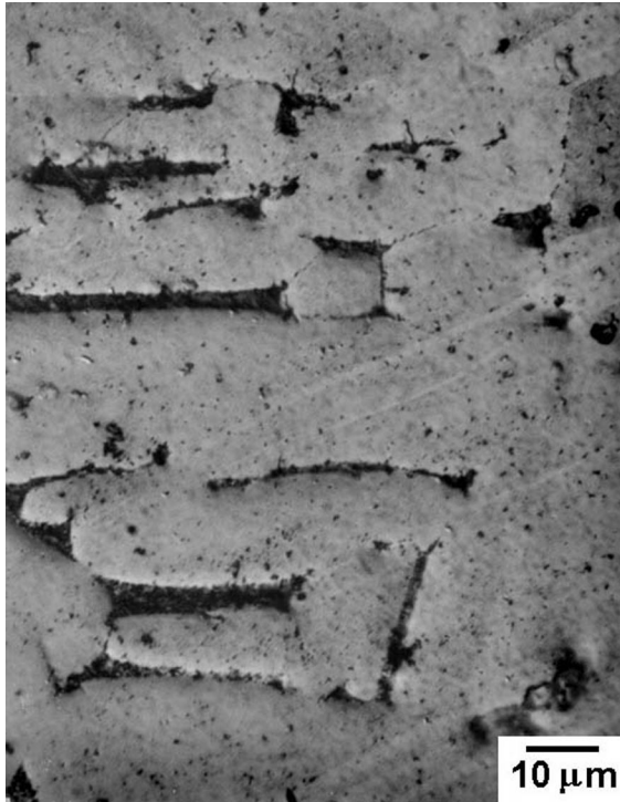
Fig. 5. Interference-contrast optical micrograph of W2 cladding after \beta\text{S-}834(18)\text{F} heat treatment. Also typical of any \beta\text{S-}T(t)\text{F} microstructure where fan-cooling preceded the (\alpha + \beta + \chi)/(\alpha + \chi) transformation.
